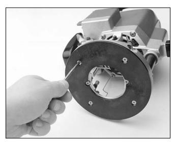
Figure 11. Removing sub-base from router.
